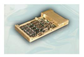
MAG's Latching Rotary-Field Ferrite Phase Shifters combine the best of phase shifter technologies. Latching Rotary-Field Ferrite Phase Shifters offer true modulo-360 degree operation with excellent peak and average power handling capabilities across a 1 GHz bandwidth at X-Band. The Latching characteristic eliminates the need for holding current thereby reducing system power needs.
